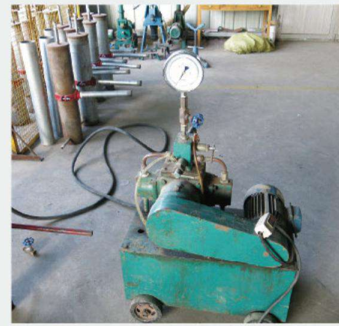
Pressure Testing Machine
